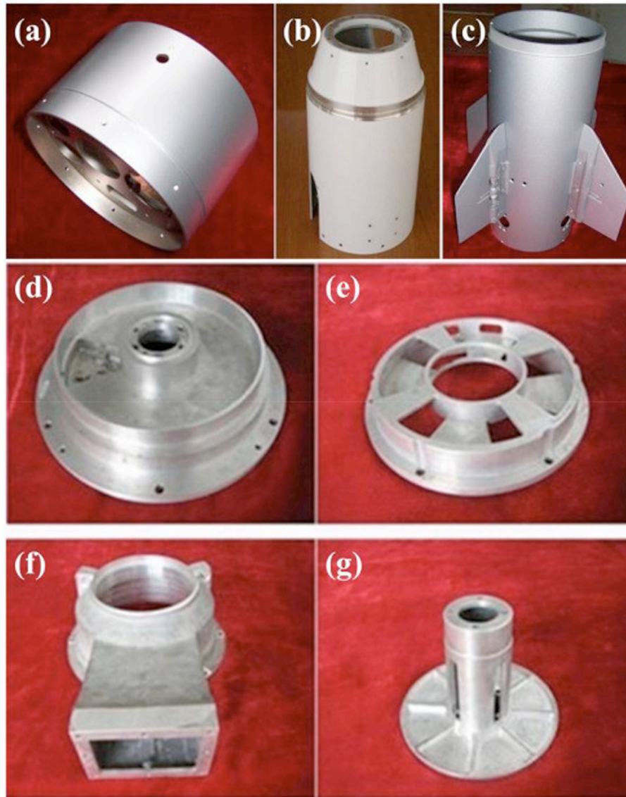
Fig. 21. Different spherical parts (a-c) missile shells (d-g) components for radars, fabricated JDM1 and JDM2 alloys. Reproduced with permission from Elsevier [235].
