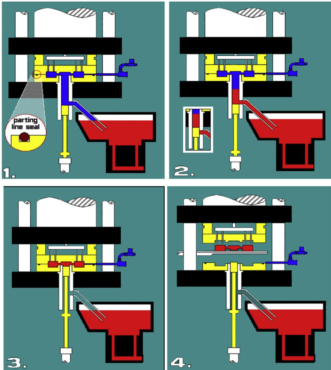
Fig. 7. Gibbs vertical vacuum assisted die casting process (Courtesy of Gibbs Die Casting, Henderson, KY, USA [11]).
