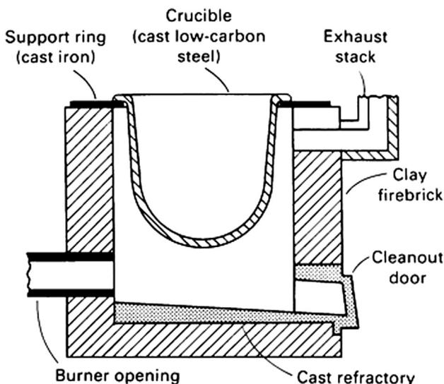
Fig. 1. Cross section of a stationary fuel-fired furnace used for the open crucible melting of magnesium alloys [2].
