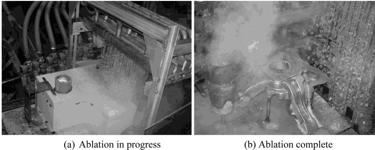
Fig. 13. Ablation casting process for aluminum and magnesium casting [26].
