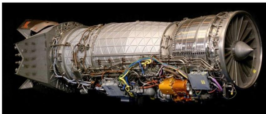
Fig. 14. Pratt & Whitney F119 auxiliary casing in ELEKTRON WE43 alloy [37].
