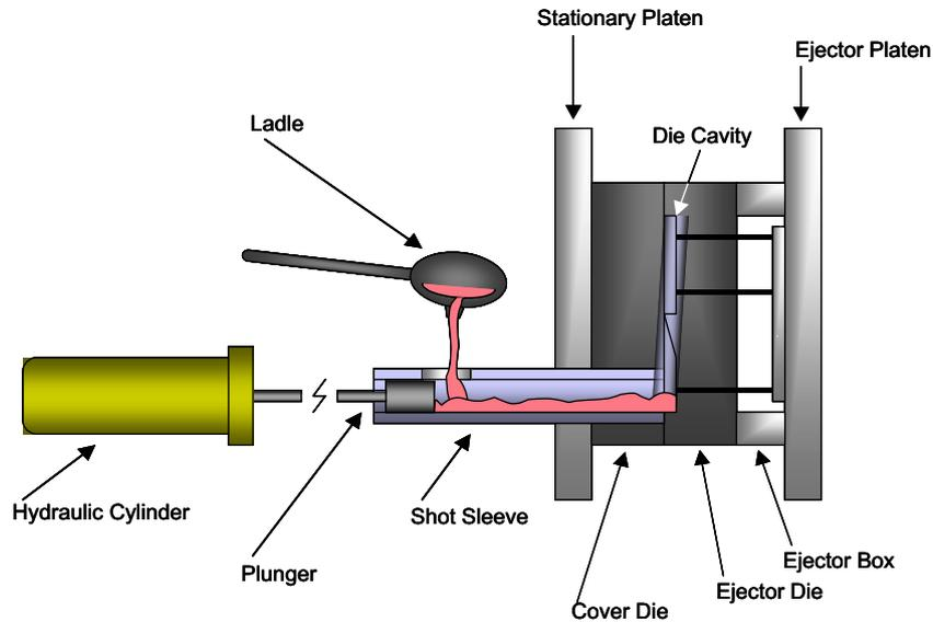
Fig. 5. Schematics of cold chamber die casting [8].
