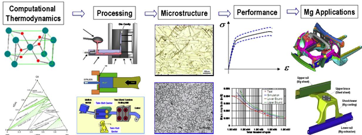
Fig. 22. Integrated Computational Materials Engineering (ICME) framework for magnesium applications.
