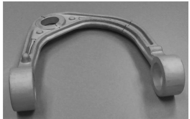
Fig. 9. A prototype magnesium control arm made by GM using low pressure die casting process.
