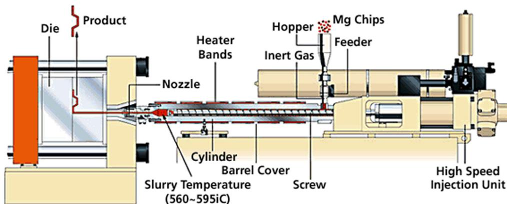
Fig. 10. A schematic diagram of a Thixomolding machine [21].
