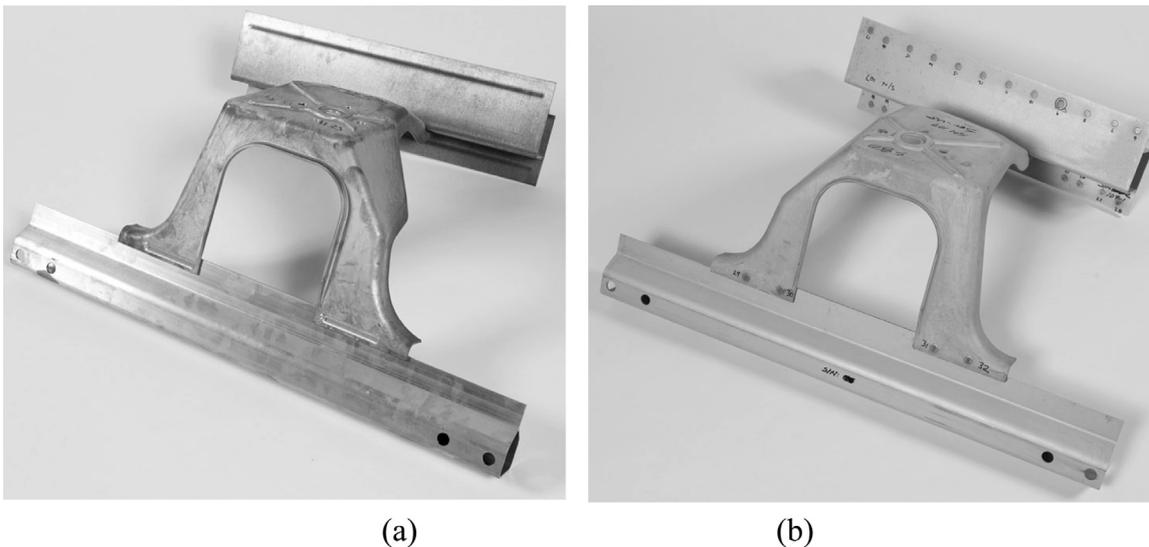
Fig. 21. USCAR demo structure build using (a) FSLW (friction stir linear welding); and (b) LSPR (laser-assisted self-pierce rivet) joining processes [67].
