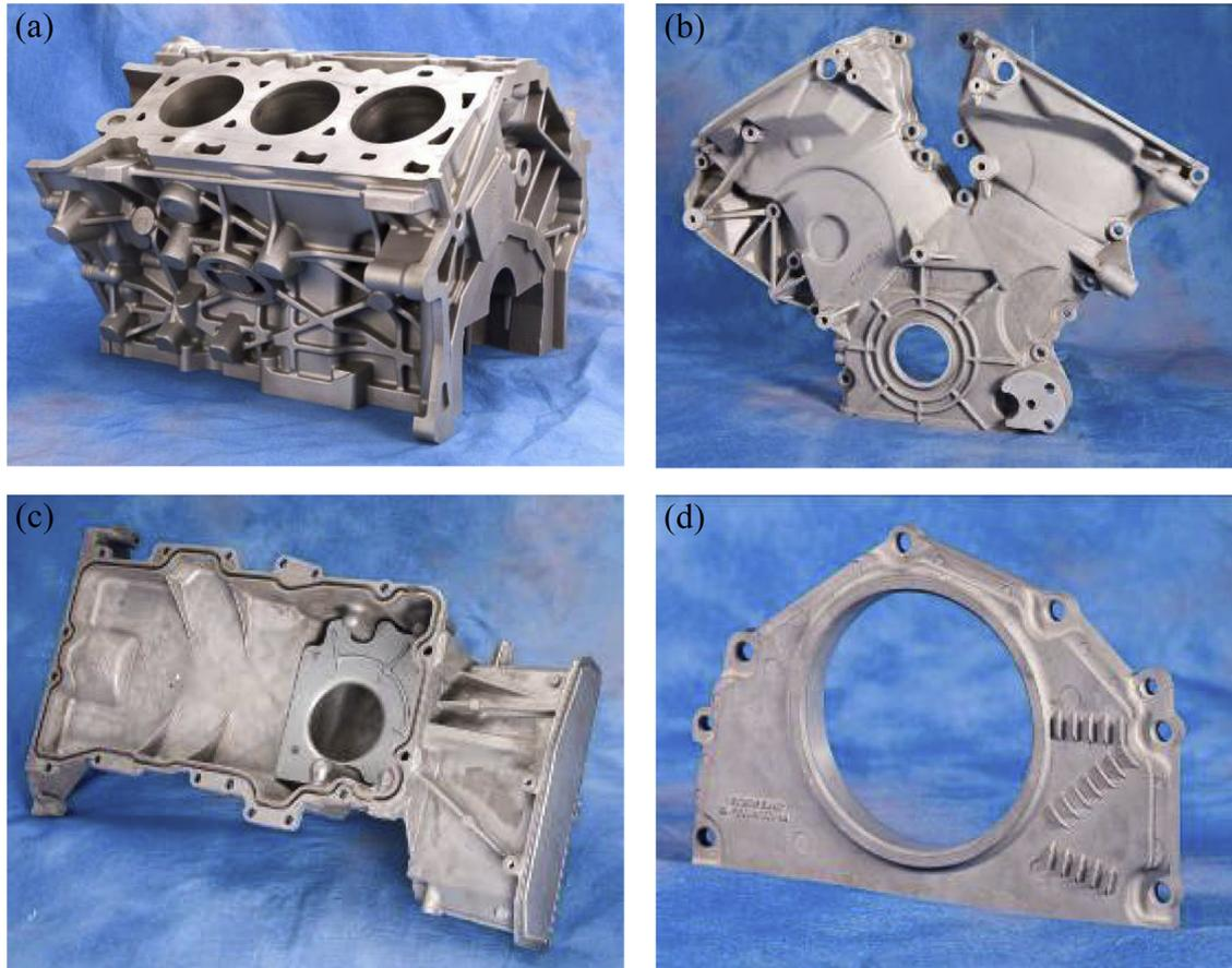
Fig. 19. Magnesium powertrain components from the USCAR magnesium powertrain cast components project; (a) LPDC cylinder block, (b) Thixomolded front engine cover, (c) HPDC oil pan and (d) HPDC rear seal carrier [54].
