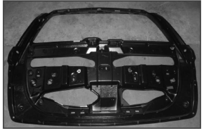
Fig. 16. HPDC magnesium casting Lincoln MKT liftgate inner (photo courtesy of Meridian Lightweight Technologies) [49].
