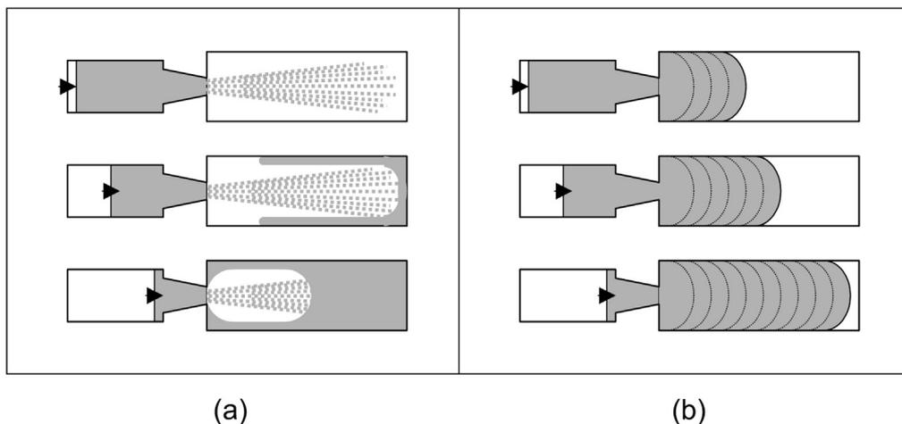
Fig. 12. Schematic illustrating metal flow in (a) conventional die casting; and (b) indirect squeeze casting process [8].
