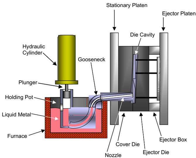
Fig. 3. Schematics of hot chamber die casting [8].
