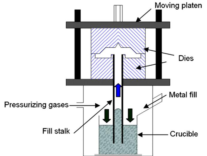
Fig. 8. A schematic diagram of a typical low pressure casting machine [17].
