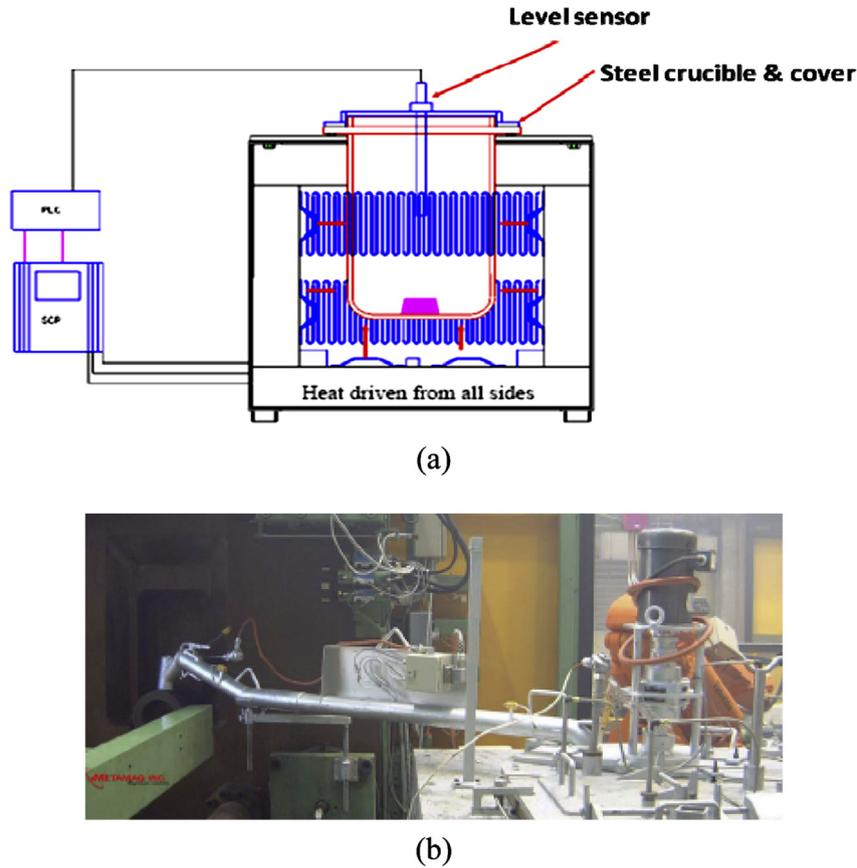
Fig. 2. (a) Modern electrical furnace with a steel cover; and (b) metal transfer tube delivering molten magnesium to a die casting machine (Courtesy of Metamag, Inc., Strathroy, ON, Canada).
