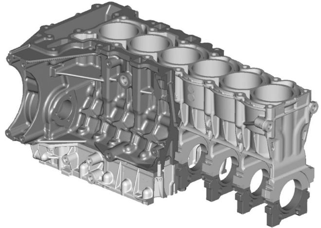
Fig. 18. The BMW composite engine block showing a cutaway of the magnesium exterior revealing the aluminum interior [35].
