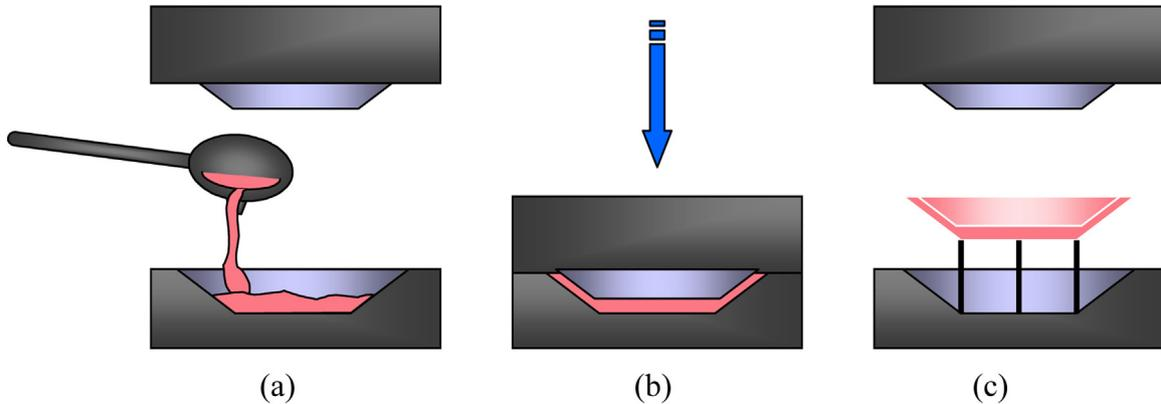
Fig. 11. Schematic illustrating direct squeeze casting process operations: (a) melt into die cavity; (b) close tooling, solidify melt under pressure; and (c) eject casting [8].
