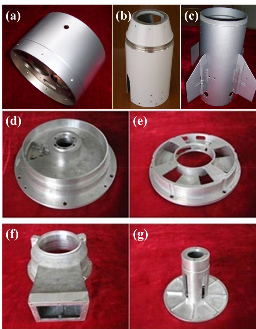
Fig. 25. Light missile shell (a ~ c) prepared by JDM2 Mg-RE alloy and radar components (d ~ g) [116].
